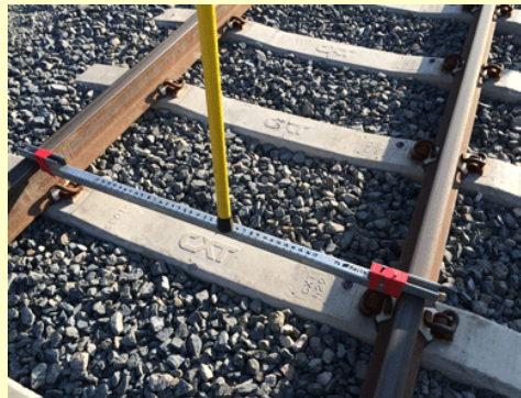
10. Reminiscent of the old "plumb bob" days with simple trolley wire, this is the technique used to measure such offset.
