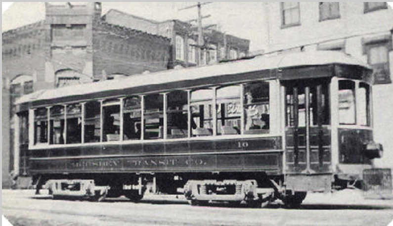
5. Hershey Transit Co. Arch Roof Car 10 with high speed trucks.
